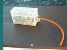
Modified Whitlock-Vibert box used for sampling fine sediment
